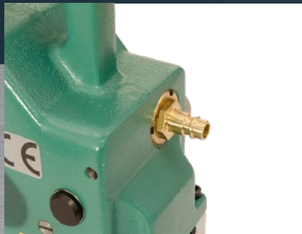
Air connection for motor and magnet
